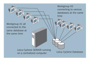
Simultaneous multi-user access to network shared databases provides optimal flexibility and project productivity. Huge point cloud databases are maintained in a simple, secure and centrally managed location.
